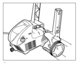
Step 1 Slide each of the mobile adapter brackets to the pressure washer. Align the pegs and holes on the brackets. Insert the 4 screws and tighten as shown.
